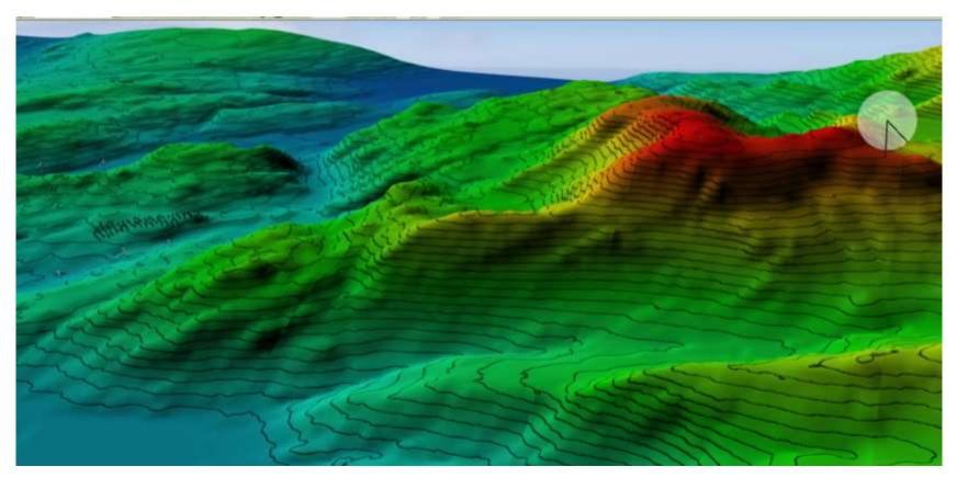
Digital Elevation Map (DEM) layers can detect changes in elevation based on the resolution. For 30 meter resolution, the contour lines are spaced 30 meters apart.
