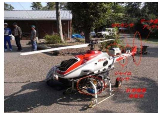
Auto-pilot RC helicopter for remote sensing
